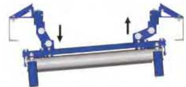
The belt conductor has guided the belt back on track.
